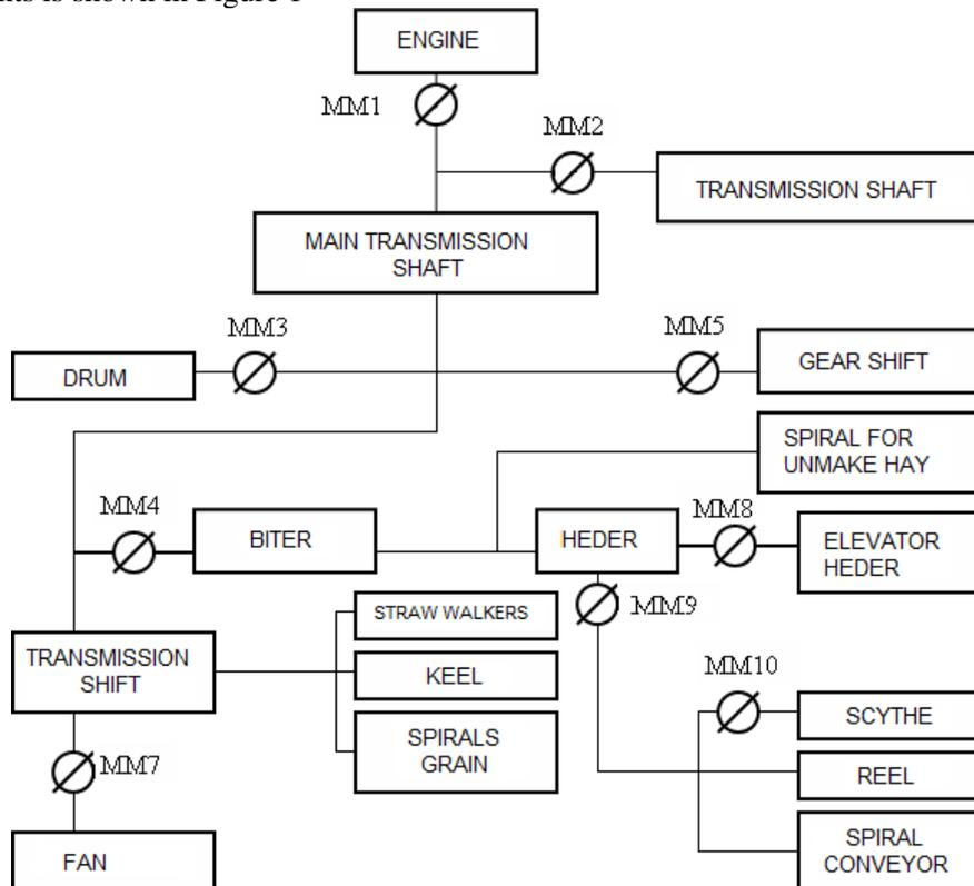
Figure 1: Measurement points for balance measurements [2]
