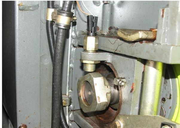
Figure 4: Inductive sensor speed elevators header, [1]
