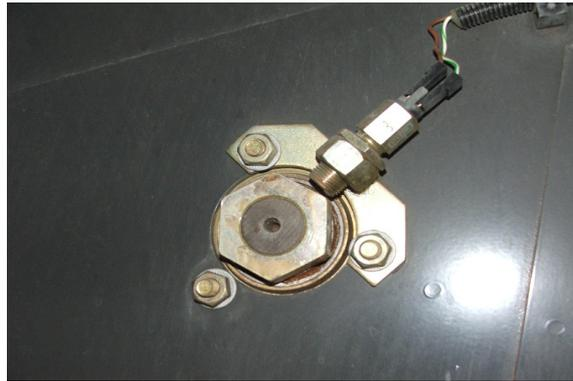
Figure 6: Inductive sensor crank rotation speed straw walkers and returned back straw spreader, [1]
