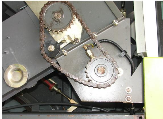
Image 8: Inductive sensor speed elevators and a spiral transporter to return unmake grains in make apparatus, [1]
