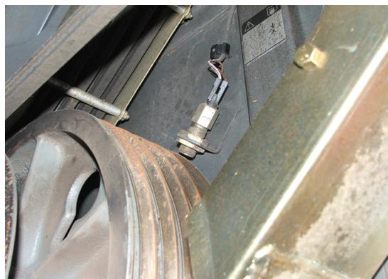
Figure 5: Inductive speed sensor repulsive biter, [1]
