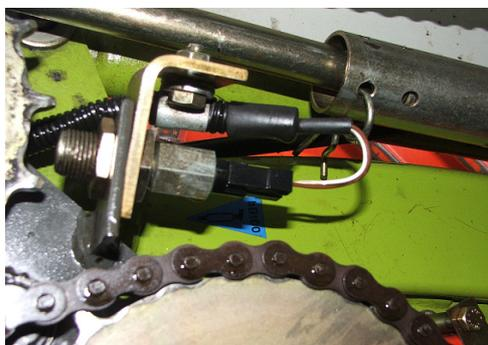
Figure 3: Inductive sensor rotation speed reel, [1]
