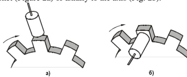
Figure 2: Installation of cylindrical inductive proximity sensor:
